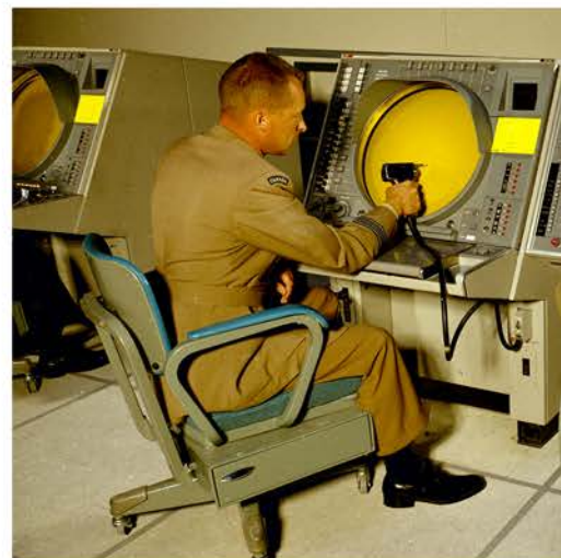
An air defence technician uses his light gun to select a target on his screen.
