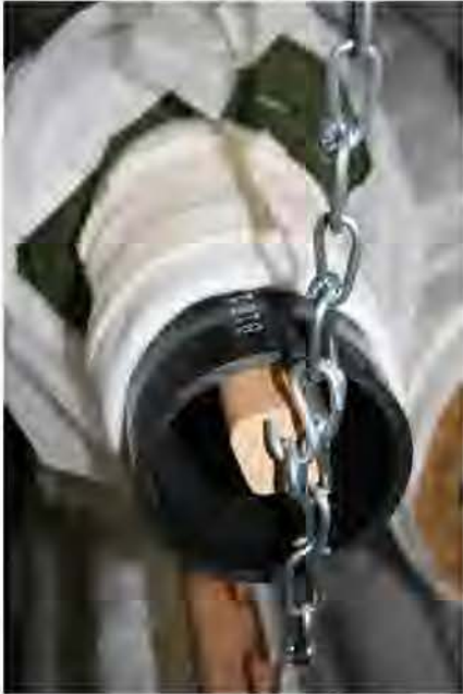
Rolled storage with ABS pipe and barrier material visible
