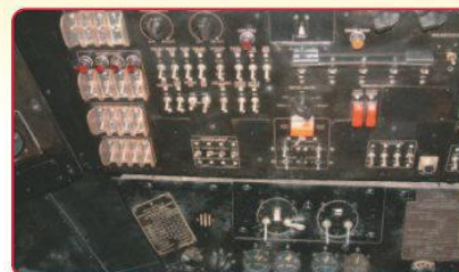
Avionic Panel with Radium Toggles, Stencilling and Dials.
